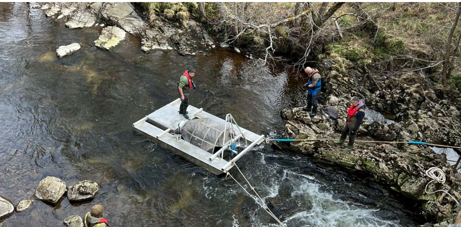
Above: The Rotary Screw Trap being deployed on the River Truim to catch salmon smolts as part of the Moray Firth Tracking Project. (Photo: Roger Knight, SFB Director).
